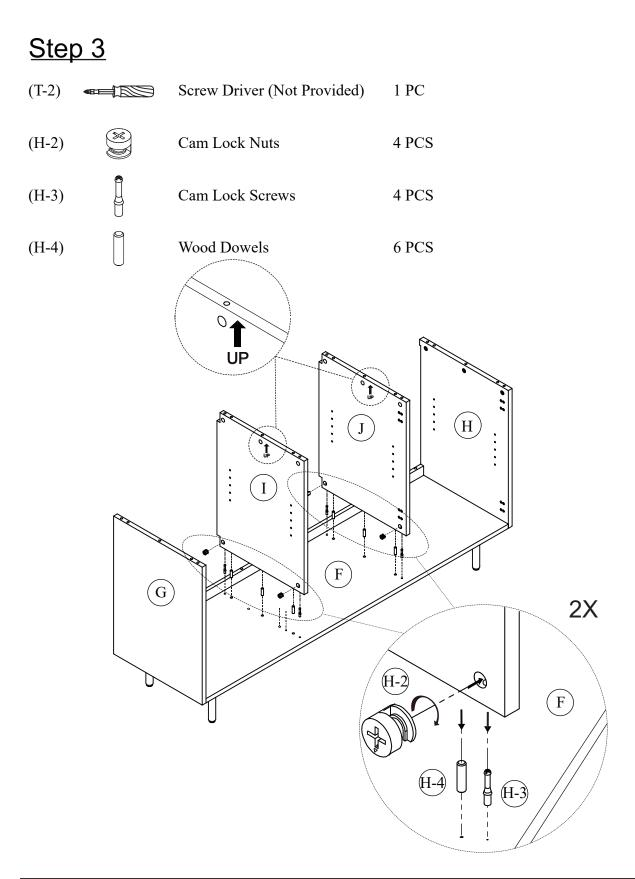
Install Cam Lock Screws (H-3) first, then insert the Wood Dowels (H-4) on the Bottom Panel (F). Fit the holes in the edge of the Left and Right Divider Panels (I&J) over the Cam Lock Screws (H-3) and Wood Dowels (H-4). Install Cam Lock Nuts (H-2) and tighten by turning clockwise using Screw Driver (T-2). Must follow Cam Lock Nuts (H-2) position before tighten.
