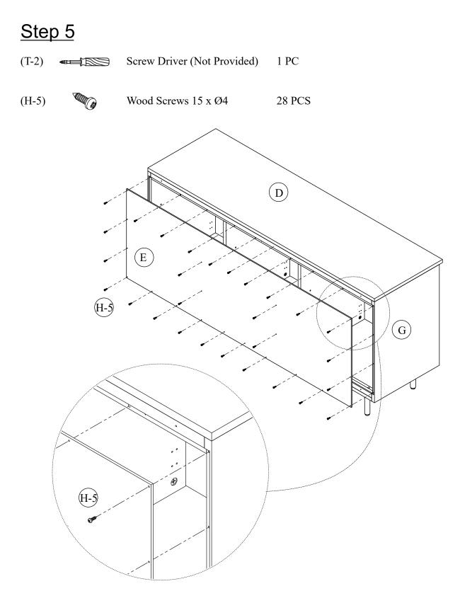
Attach Back Panel (E) into pre-assembled unit (Step 4). Secure using Wood Screws (H-5) and fully tighten by a Screw Driver (T-2).
