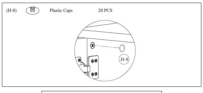
Attach Plastic Caps (H-8) into the holes of Cam Lock by hand.
