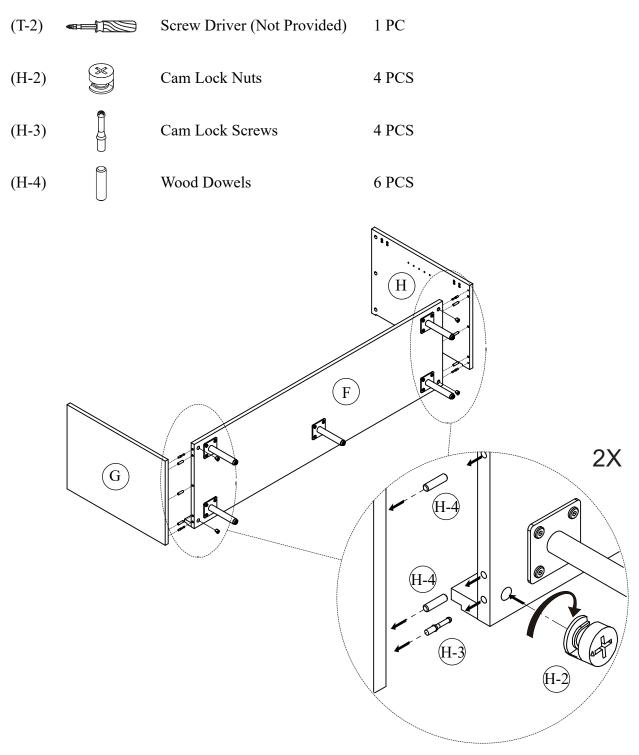
Install Cam Lock Screws (H-3) first then insert the Wood Dowels (H-4) on the Left and Right Side Panels (G&H). Fit the holes in the edge of the Bottom Panel (F) over the Cam Lock Screws (H-3) and Wood Dowels (H-4). Install Cam Lock Nuts (H-2) and tighten by turning clockwise using Screw Driver (T-2). Must follow Cam Lock Nuts (H-2) position before tighten.
