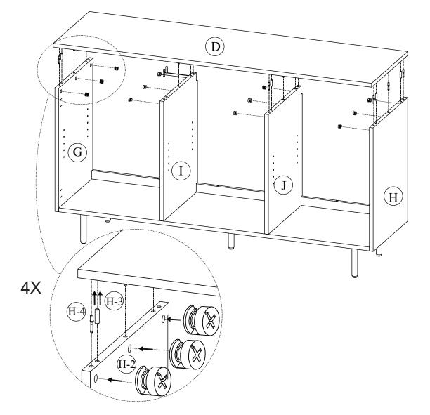
Install Cam Lock Screws (H-3) first, then insert the Wood Dowels (H-4) on the Top Panel (D). Fit the Cam Lock Screws (H-3) and the Wood Dowels (H-4) on the Top Panel (D) to the holes in the edge of the Left & Right Side Panels (G&H) and Left & Right Divider Panels (I&J). Install Cam Lock Nuts (H-2) and tighten by turning clockwise using Screw Driver (T-2). Must follow Cam Lock Nuts (H-2) position before tighten.
