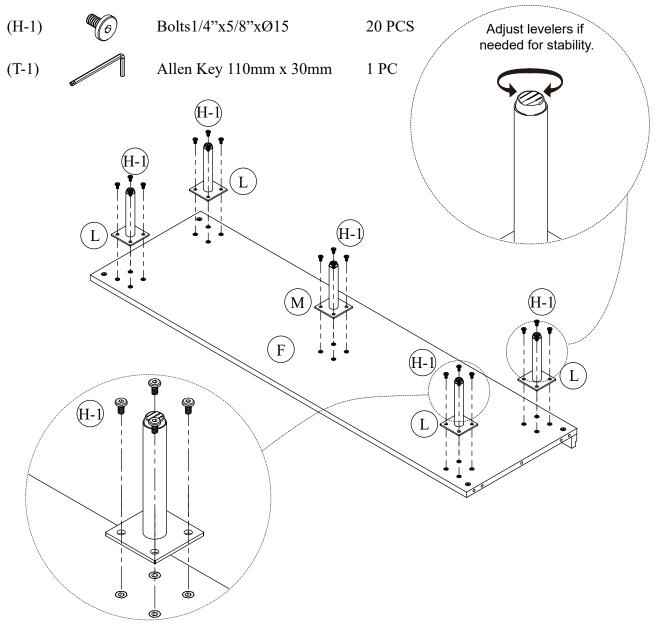
Position Metal Legs (L) and Middle Metal Leg (M) to corners and the center of Bottom Panel (F); Secure by using Bolts (H-1) and fully tighten all bolts by Allen Key (T-1).
