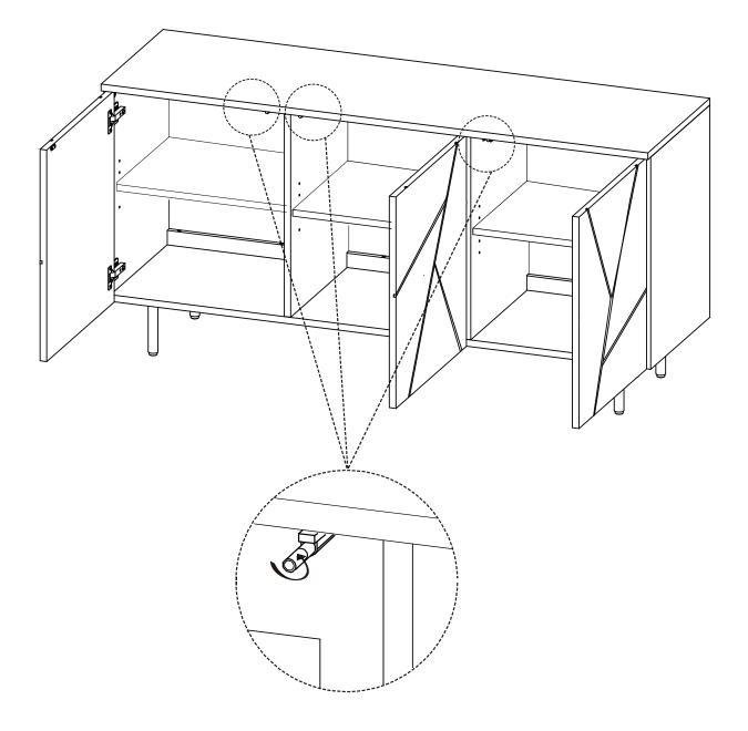
If any door failed to close properly, adjust the length of the magnetic latch's pin by turning it counterclockwise, as shown. The push pin's length will extend to allow the lock to engage. You will hear a soft click. Door will close.
