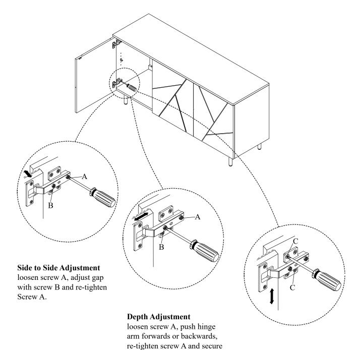
**Height Adjustment** loosen screw C, adjust door height and re-tighten screw C.
