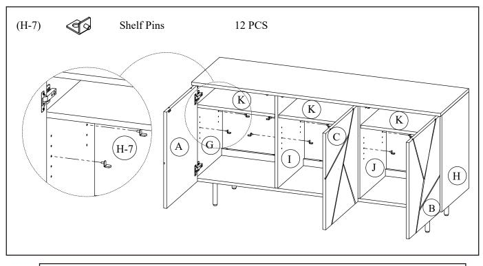
Insert Shelf Pins (H-7) into Left and Right Side Panels (G&H) and Divider Panels (I&J). Then insert Adjustable Shelves (K) into assembled unit.
