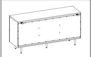
Using a second person to assist you, place the unit in the desired final location against a wall. It is suggested to use a stud finder to find wall studs along the length of the unit and roughly 1 inch below the top of the unit. Where possible, mark a drill hole position on the wall where there is a stud and Screws (02) in the location of the wall studs.
